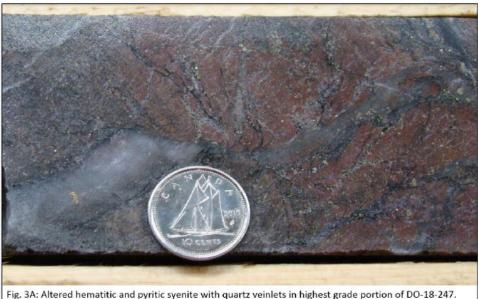
Fig. 3A: Altered hematitic and pyritic syenite with quartz veinlets in highest grade portion of DO-18-247. Note speck of visible gold to the left of the dime.
