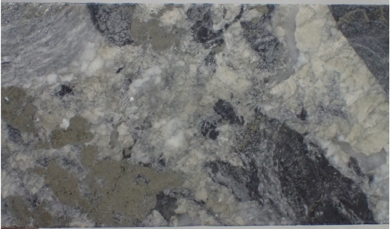
Plate 2: Pyrite-Fe Carbonate-(quartz) zone at 2,045.7 m in TB-23-003W2, within interval grading 6.4 g/t Au. NQ core, 47.6 mm diameter.
