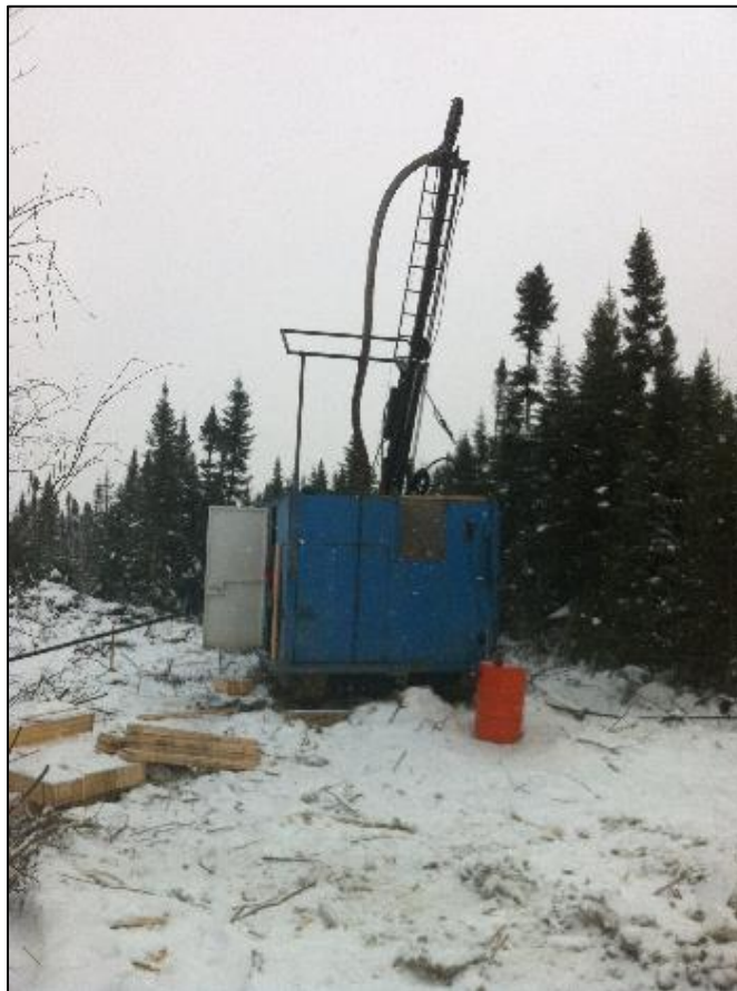
Figure 10.1 Diamond Drill Rig Set-Up on a Drill Hole at the Douay West Deposit (December, 2016)
