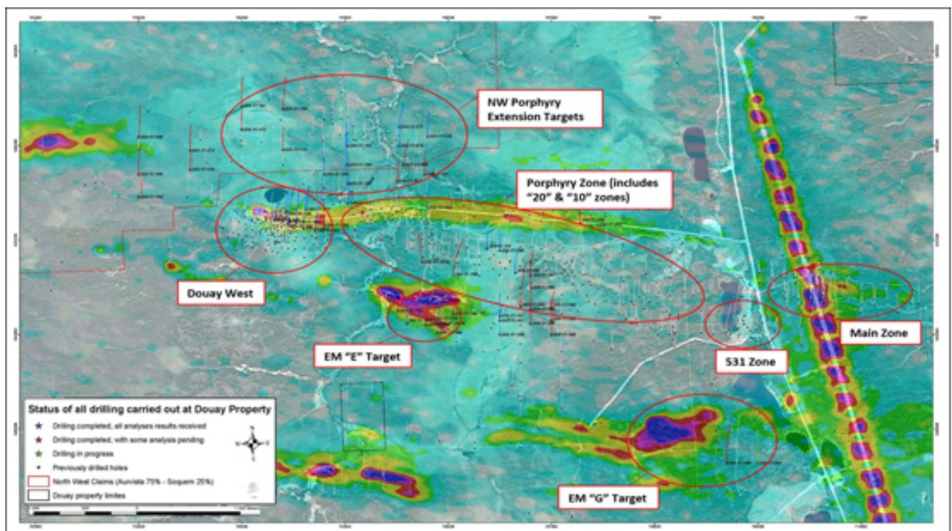
**Figure 1: Drill-Hole Location Map with EM Targets**
