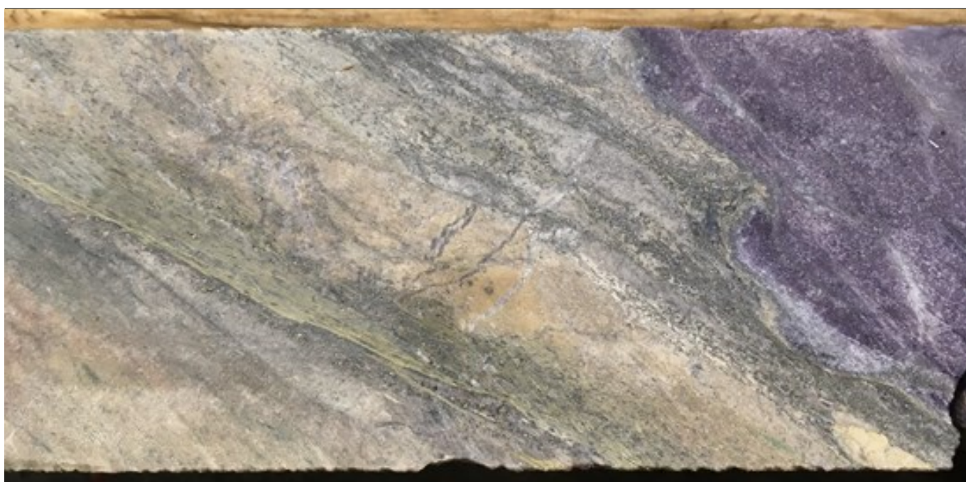
Fig. 3: NQ core (47.6mm diameter) from 41.3-41.9m in DO-20-272A, which assayed 13.25 g/t Au. Note yellow sericite defining foliation, stronger Fe-carbonate (pale orange color) and relatively abundant fine disseminated and stringer pyrite, as well as purplish grey fluorite-carbonate injection in upper right part of photograph.
