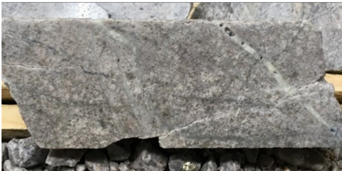
Fig. 3: NQ core (47.6mm diameter) from 203-204m downhole in DO-20-283; that interval assayed 5.25 g/t Au. Both disseminated and veinlet pyrite are present in bleached syenite. Photo is of a selected interval and is not necessarily representative of all mineralization hosted on the property.
