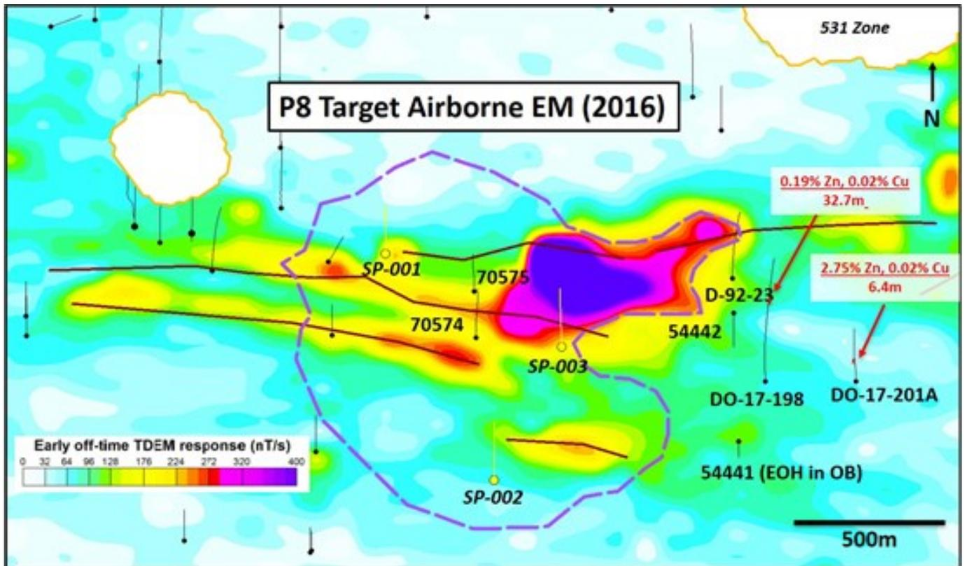
**Fig. 2 & 3: P8 Target (purple dashes) defined as combined and overlapping 2016 airborne EM conductor (Fig. 2, above) and 2020 chargeability anomaly at 300 m depth (Fig. 3, below). Solid brown lines represent historical INPUT conductor axes. SP holes are currently being permitted.**
