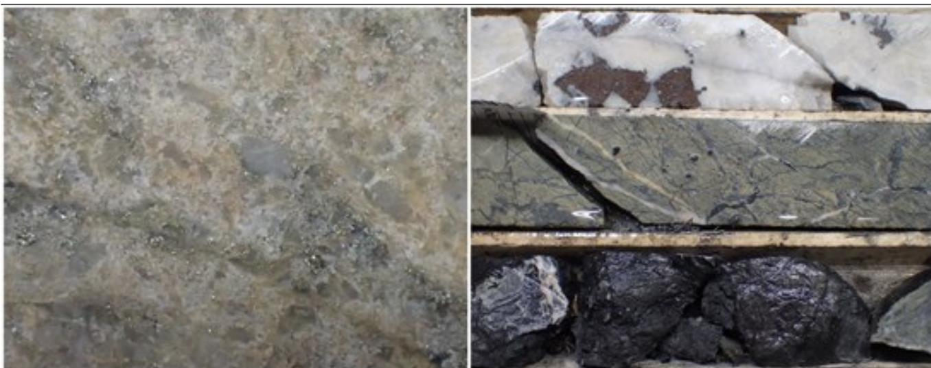
**Fig 4: Left, new mineralization style from historical hole 70575, beginning at top of bedrock: pyritic quartz breccia in thickened interflow sedimentary/exhalite horizon. Right, core from historical hole DO-17-201A: another new mineralization style including white carbonatitic injections with coarse brown sphalerite in strongly graphitic black interflow sediments and sericite-Fe-carbonate (paler green) altered volcanics.**
