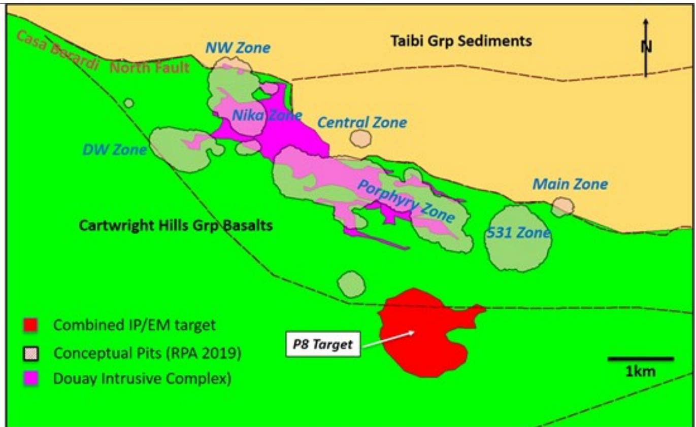
**Fig. 1: Location map for the new P8 Target. Note scale of this target relative to different resource zones. Syenitic bodies with associated (proximal) gold mineralization are present at the Nika and Porphyry Zones, while more distal mineralized zones such as Douay West (DW) and 531, and including the P8 Target area, are characterized by stronger structural control and spatial association with sedimentary horizons within a predominantly basaltic sequence.**
