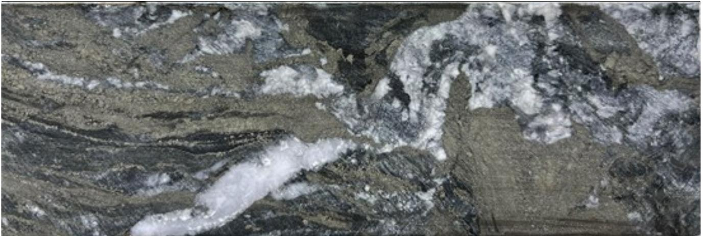
**Plate 1:** Eagle-Telbel style semi-massive pyrite with irregular and broken up iron carbonate veinlets from 346.5 m in EM-22-005, part of 1 m sample grading 1.2 g/t Au.
