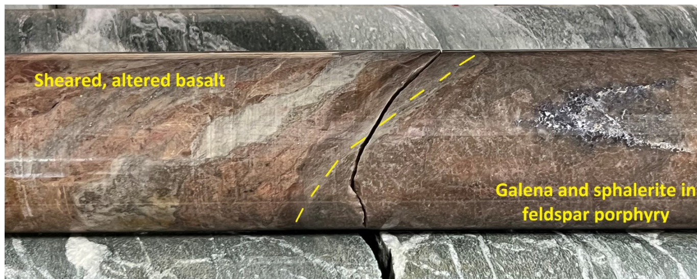
Plate 2: Drill hole DO-23-326W1 showing sharp contact at ~1,360 m between sheared basalt and feldspar porphyry; both lithologies are strongly altered by hematite, albite, K-feldspar, carbonate, silica and sericite. Note the presence of galena and sphalerite in a flat fracture near the contact.
